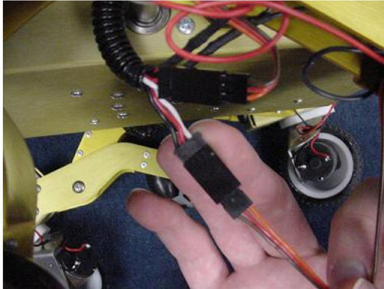
3. Thread the new servo wires back through the leg in the same way as the servo you just removed. Connect the servo, making sure to align the brown and black wires. Tuck all of the wires carefully back in to the leg and secure with zip ties. Try to keep the wires and zip ties tucked inside the leg as much as possible. This will keep the center omni wheel from hitting the wires.
