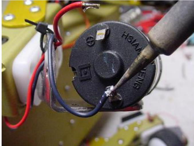
3. Unsolder the black and red wires from the motor and remove the motor. Thread the tips of the wires in to the leads on the new motor and solder in place. Note that the red wire connects to the positive pole and the black wire connects to the negative pole.
