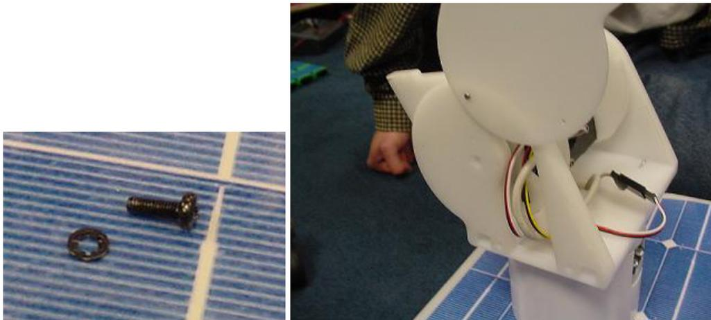
10. If you are installing a new style (black) servo, remove the washer from the screw that secures the servo horn to the servo. Align the next plastic head layer and fit the servo horn on to the servo. The head should be level at this point. Secure with the screw making sure that the screw is tight. This takes longer than expected. Keep turning until the screw is tight.
