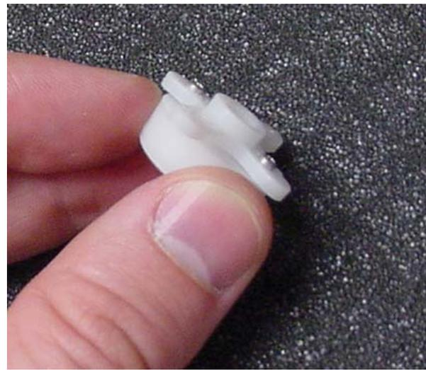
7. In order for the servo horn to fit, we need to trim the pieces of the horn which protrude outside of the circle of the coupler.
