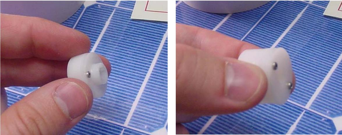
In either case, we need to separate the two pieces of the coupler. These screws require the T5 driver. Make sure to save the screws we removed, we will need them later.
