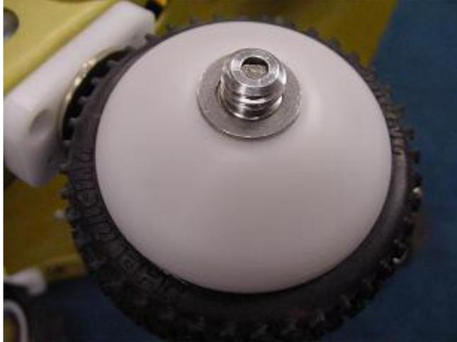
5. Fit the wheel back in place. Wiggle the wheel to verify that it is completely seated. Replace the washer and fasten with the bolt.
