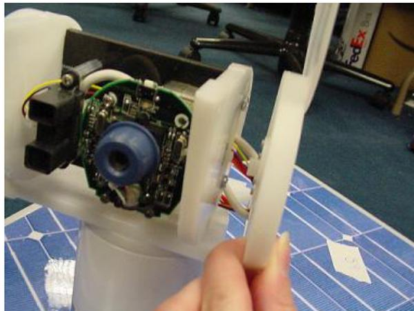
3. Separate the outer panels and servo horn from the head.
