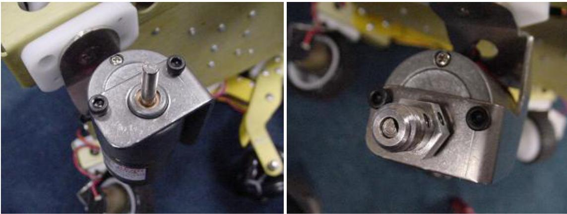
4. Replace the two black screws holding the motor to the metal angle. Fit the aluminum hub on to the motor shaft so that the set screws will be aligned with the flat side of the shaft. Tighten the set screws using a drop of loctite 242 to keep them secure. Make sure the set screws are firmly against the motor shaft flat.
