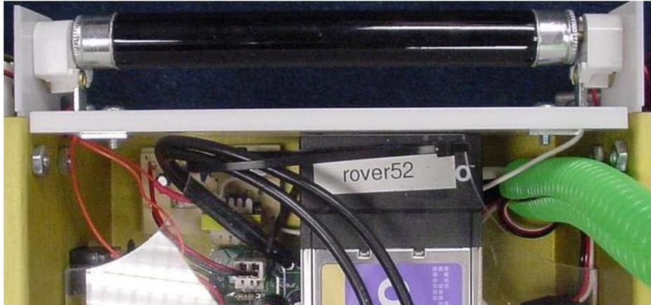
6. When you replace the clear plastic panel inside the rover, the green tubing should go through the front right hole and the power cable to the battery pack should go through the front left hole. The power cable should then be zip tied to the plastic panel so that pulling on the cable will not stress the cable's connection to the power board inside the rover.
