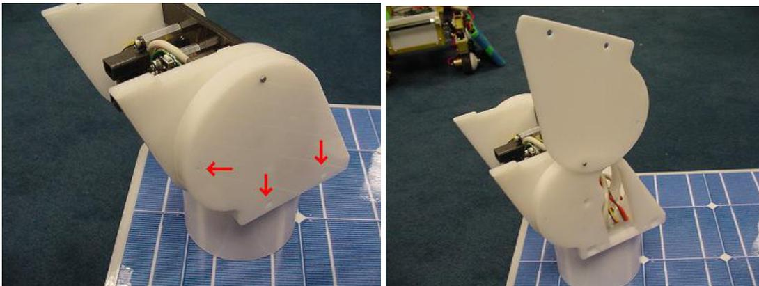
4. Remove three of the four screws on the left side of the rover's head. You will need a T5 torx wrench. Swing the outer layer of plastic out of the way. Both ends of the camera are now free and the camera can be removed.
