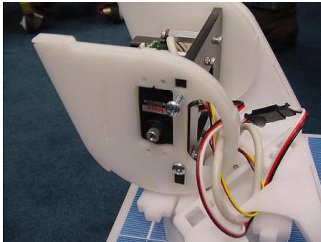
8. Reattach the inner most plastic layer to the rover's head with two screws.
