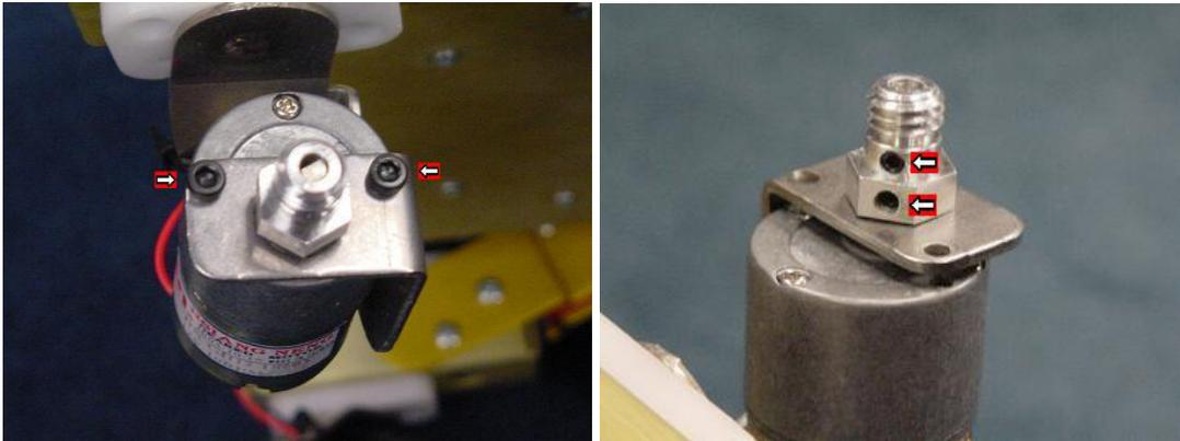
2. Remove the two black screws on either side of the motor. Loosen the two set screws that hold the aluminum hub on the motor shaft flat, and pull the aluminum hub off the motor shaft.
