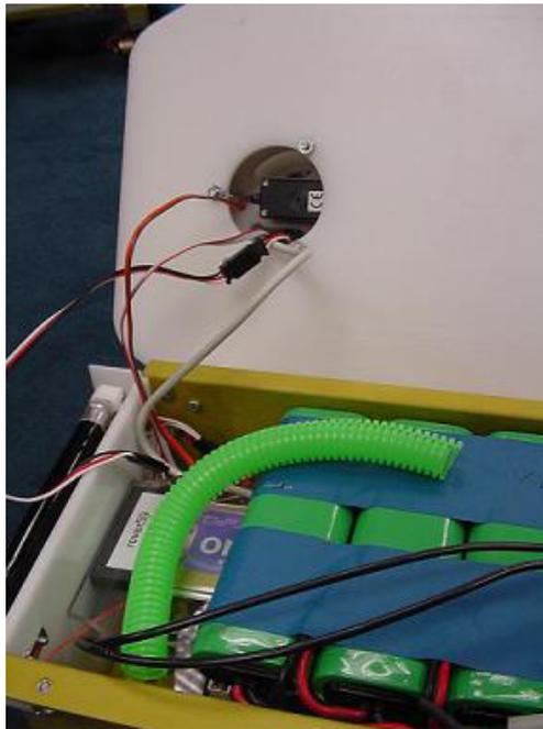
12. For the new style servos, there will be enough slack in the wires for the connector to fit inside the robot rather than sit at the back of the robot's head. Open the rover and remove the green tubing. Pull the connector down through the neck of the robot and then replace the tubing.
