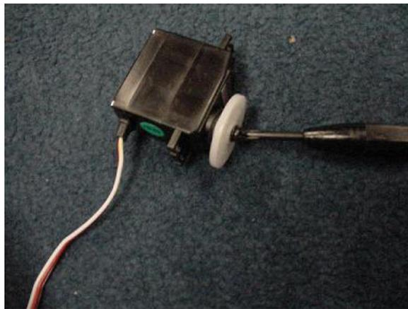
5. Remove the screw holding the servo horn on the replacement servo.
