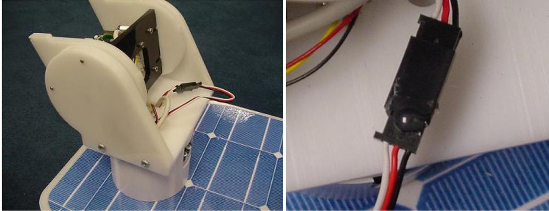
11. Secure the outer head layer with the three remaining screws. Pull any excessive slack in the servo wire to the back of the head, but be sure that the head still has full range of motion without putting tension on the wires. Use a small dab of hot glue to make sure that the servo does not come unplugged.
