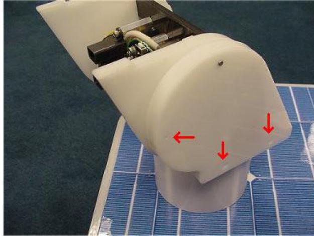
1. Remove the rover's head cover. Then remove three of the four screws on the left side of the rover's head. You will need a T5 torx wrench.
