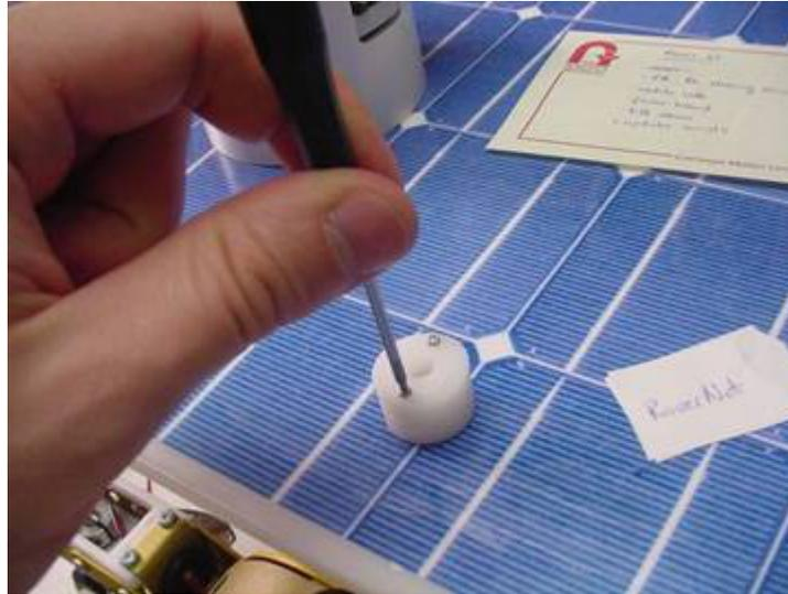
4. We now need to attach a servo horn to the lower piece of the coupler, such that we can interface the new servo with the steering shaft. We start by removing the horn which comes attached to the new servo.
