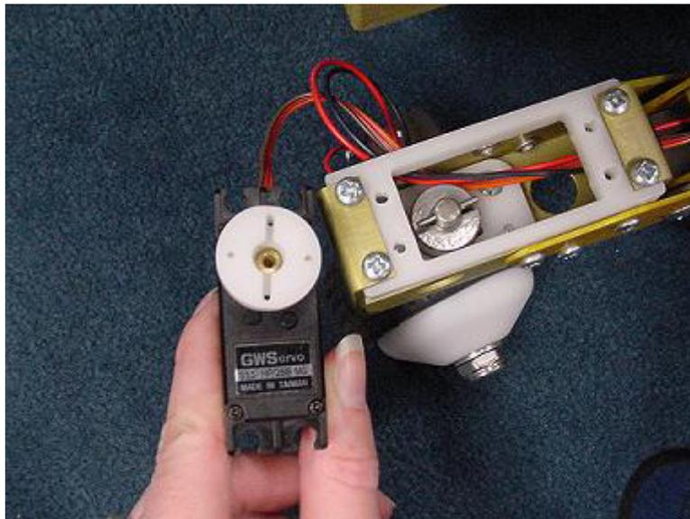
4. Turn on the rover and connect to it using the Calibration software. Load the servo calibration from the rover. Center the slider of the new servo. This is a good time to make sure that the servo works and is connected correctly. Position the servo horn on the servo as close to vertical as possible. Making sure that the wires are out of the way, replace the servo and secure the screws.
