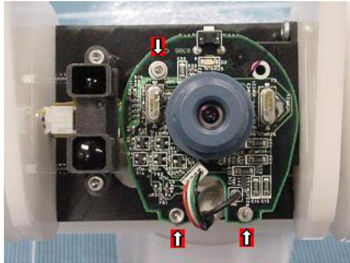
3. Remove the three screws on the front of the camera that secure the camera to the robot's head.
