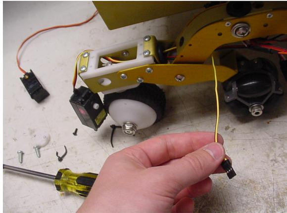
9. This new servo horn coupler combination is pressed down onto the steering shaft. The servo horn has slightly warped the coupler, so it is a tighter fit than before. It may require some force before the coupler pops into place.
