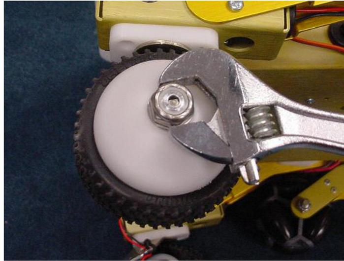
1. Remove the bolt attaching the wheel to the motor.
