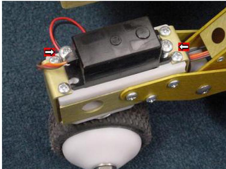
2. Cut the two zip ties that secure the wires in the rover's "legs". Unplug the servo and remove it.
