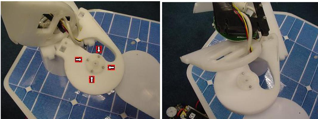
6. If you are changing from an old style servo (clear) to a new style servo (black), remove the four screws securing the old servo horn to the rover's side head panel. Use two of the screws to attach the new servo horn. This is a little difficult
