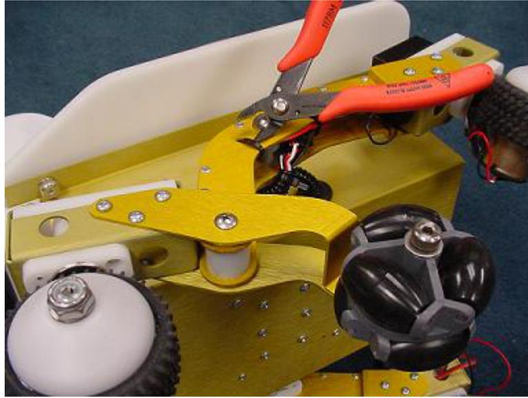
3. The white steering coupler which attached the servo to the steering shaft can be put together one of two ways. These are what they look like:
