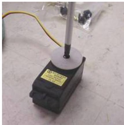
5. Next we select the cross shaped servo horn from the bag of servo accessories and insert the two screws we saved into the new horn in the two holes closest to its center. These are the holes on the shorter axis of the cross nearest the center hole. Thread the screws all the way into these holes and continue turning them, so that they strip the threads that they just cut in the plastic.
