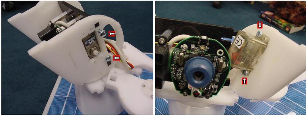
4. Remove the two screws holding the final layer of plastic in place and gently pull the plastic piece from the rover's head. Then remove the two screws securing the servo and remove it from the plastic. Unplug the servo from the servo extender and remove the servo. For old style servos (clear), the connection will probably be just behind the rover's head. For new style servos (black), the connection may be inside the rover's neck or inside the green tubing.
