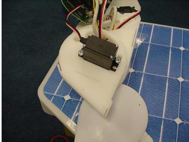
7. Thread the servo wires back through the head in the same way as the servo that was removed. The servo wires follow the same path as the camera and IR wires. Reconnect the servo and servo extender. Push the servo in to the square hole of the inner most plastic layer and secure with two screws.
