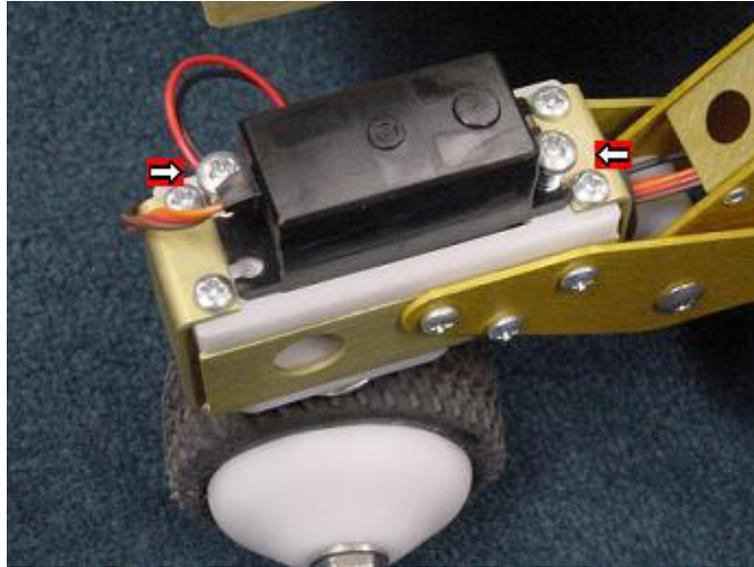
1. Remove the two screws securing the servo and then lift the servo from the rover. Make sure to remove the white servo horn as well.
