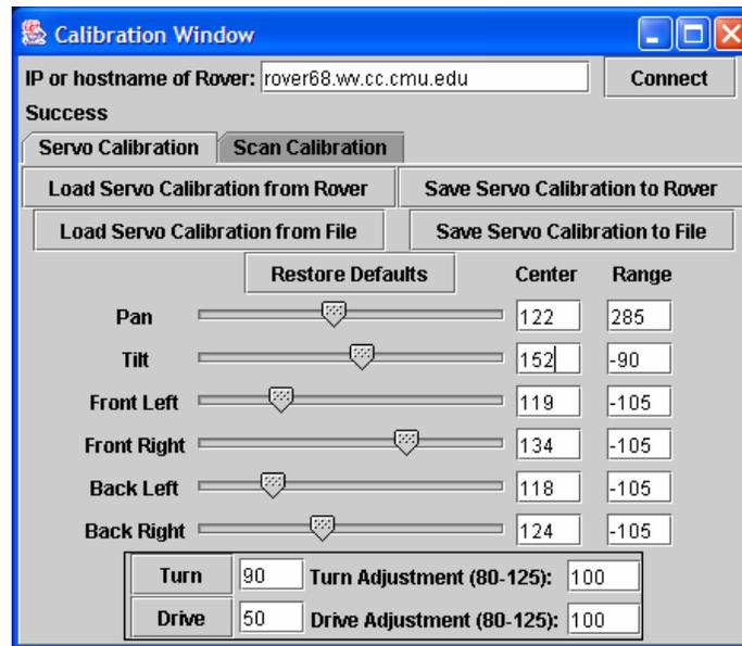
9. Turn the rover on and connect to it using the Calibration software. Load the servo calibration from the rover. Center the tilt servo slider. This is a good time to make sure that the new servo is working. For the new style servo, set the tilt servo range to -90. This is because the new all-metal gear servo moves in the opposite direction than the old style servo does.
