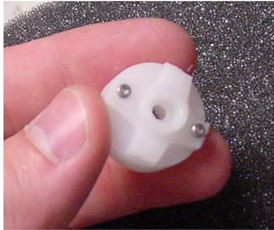
8. Now thread the wire from the new servo through just as it was in the original configuration.
