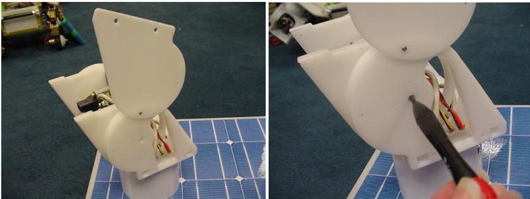
2. Swing the outer piece of plastic out of the way and remove the screw in the center of the panel underneath. This screw holds the servo horn on the servo.
